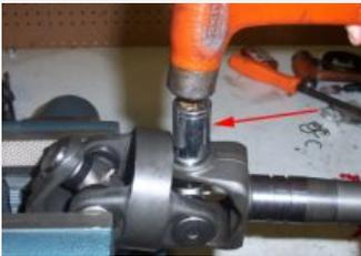
**1.3** After the clips are out, tap the u-joint one direction until you can remove the cup on the opposite side. Use a suitable socket so you do not hit the yoke with the hammer.
