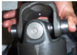
**2.3** Insert both u-joint cups while centering the yoke.
