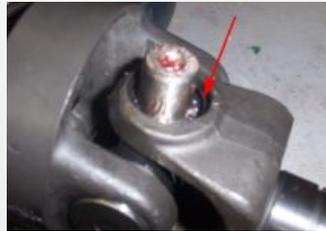
**1.4** Use a small pick or screwdriver to remove the seal if it has stuck to the u-joint.
