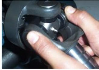
**2.5** Now with both clips in, turn the yoke and see if it turns okay. If it is stiff you can try hitting one of the u-joint cups. If it is still stiff, try hitting the opposite side. That should clear it up. Now you will need to grease the u-joints using a grease gun, and grease approved for u-joints.
