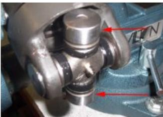
**2.1** Now with the yoke out the way we can start reassembly. Install both u-joint cups on the u-joint and check to make sure they rotate smoothly. Then if all is okay, take them off. If it rotates rough, most likely it will have to be replaced.
