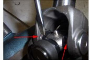
**1.2** Remove the clips that hold the u-joint together. Usually pushing on it with a screwdriver will do the trick. You may need to use a screwdriver on both sides.
