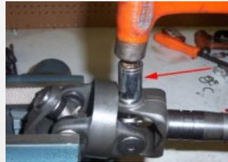
**1.5** Now, using a socket of appropriate size, pound the u-joint the other direction. The purpose of the socket is so that you don't hit the u-joint post with a hammer. You want the socket to fit over the post and to contact the body of the u-joint before the post.
