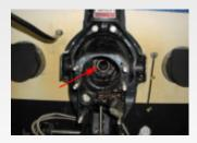
**3.1** Rotate the gimble bearing by hand. If it feels smooth it should be okay. If it is rough at all it should be replaced.
