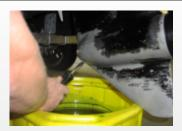
**1.2** Place a suitable container under the bottom drain plug. Remove the bottom drain plug.
