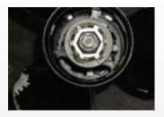
3.8 You may need to rotate the propshaft counter-clockwise as you push the stern drive on. It will aid in lining up the splines. It is best if you have the propinstalled, it will give you something to grab onto. Now install the washers and nuts that hold the stern drive on. Also torque the propnut to 50 ft. Ibs. Don't forget to bend the tab on the tab washer.
