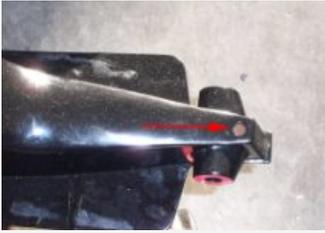
**1.1** Remove the trim tab bolt with a 3/8" Allen key. Some of the older drives may use a 5/16".
