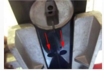
**1.4** Remove the two back locknuts. Use a 5/8" socket.
