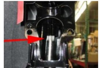
**2.4** The two halves are now ready to be put together. You may find it easier to use two people to do this. As you bring the halves together, the first thing that needs to line up is the copper water tube with the plastic tube guide.
