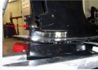
**1.3** Remove the front locknut. Use a 5/8" wrench or socket.
