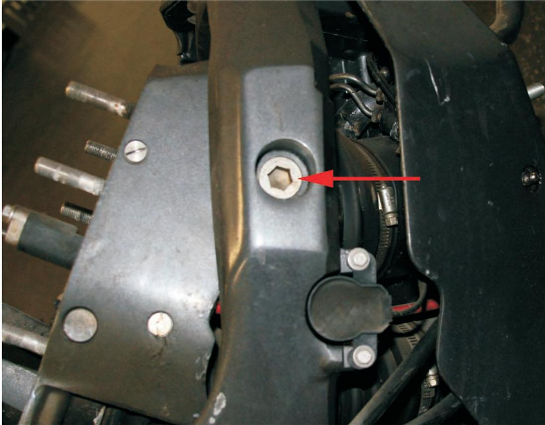
**Step 2.5:** Remove the hinge pins from both sides of the gimbal ring with a 1/2 inch allen socket and a breaker bar.
