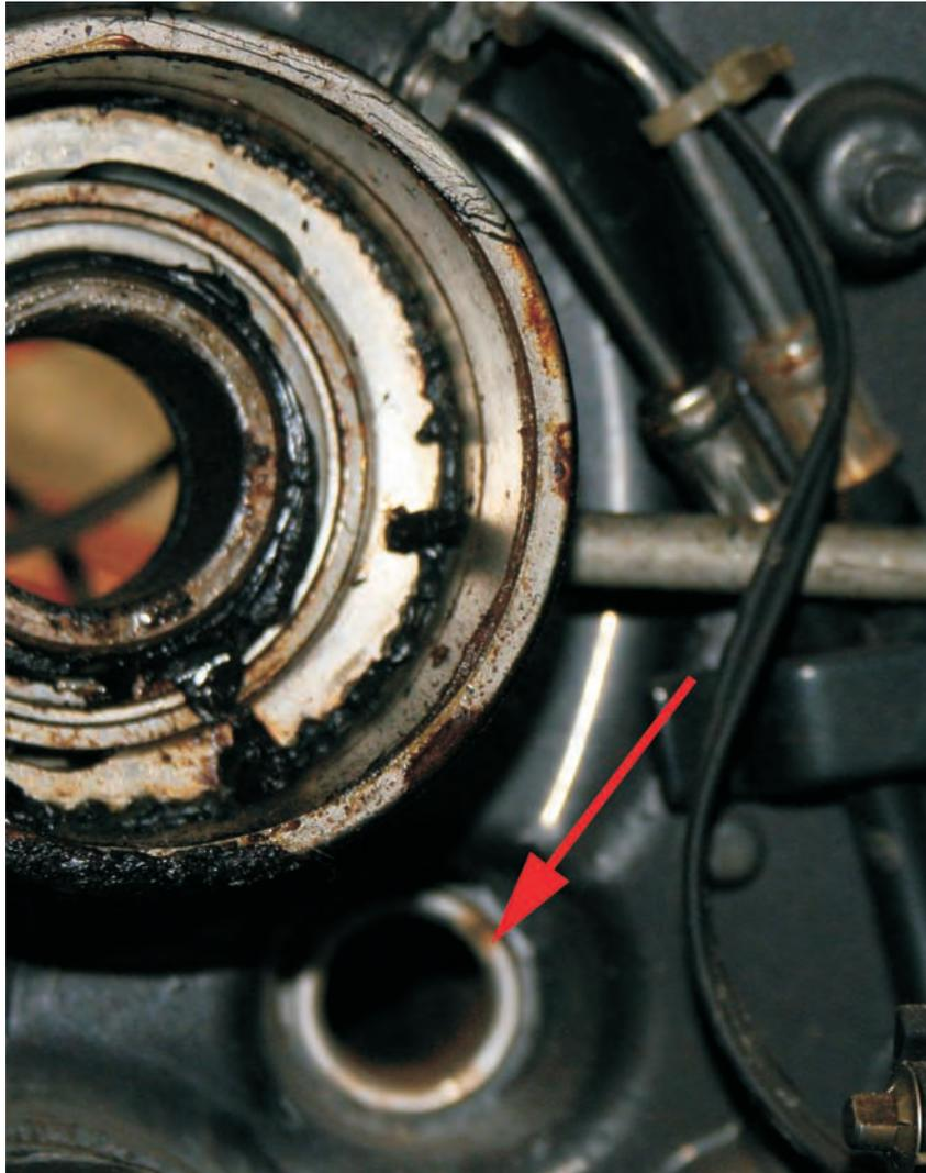
**Step 3.3:** Feed the shift cable of the new bell housing through the shift cable tube which is located just below and to the right of the u-joint bellows flange.
