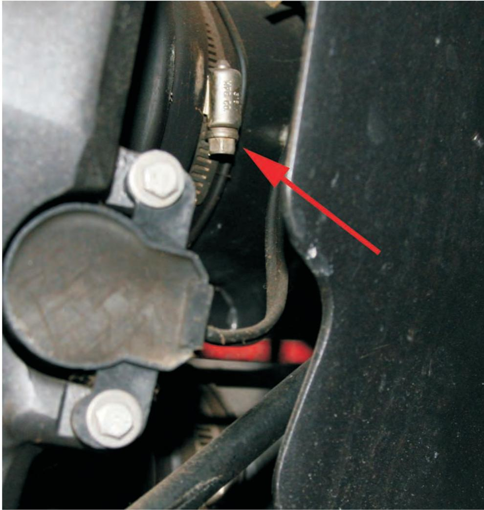
**Step 4.2:** Now you can tighten down the u-joint bellows clamp by turning the steering wheel to the left to access the clamp.
