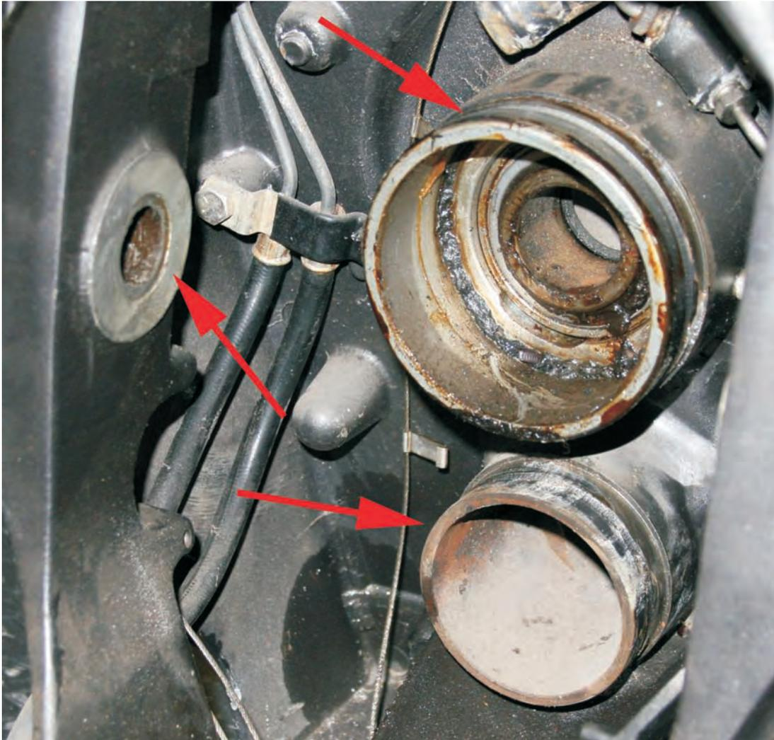
**Step 3.1:** Now you will prepare the gimbal ring to accept the new SEI bell housing. Clean the area where the plastic washers will contact the gimbal ring to remove any corrosion and also the flanges for the bellows.
