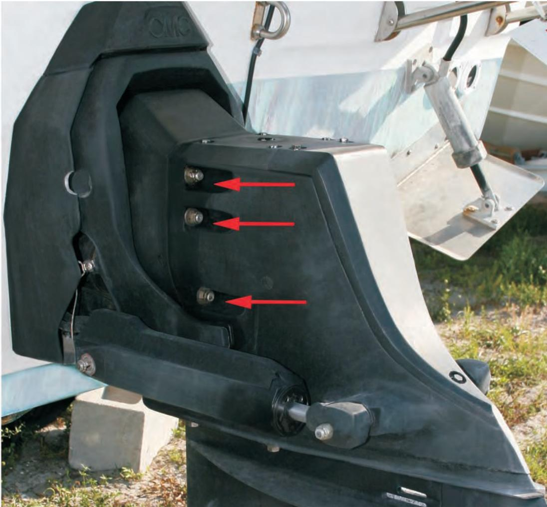
**Step 1.2:** Remove the six nuts and washers holding the upper unit to the bell housing. Once this hardware is removed the drive will be ready to remove. Simply pull back on the drive to remove it. If it is stuck you can tilt the unit up by hand and place a 2x4 between the drive and the transom assembly. Then let the drive rest on the 2x4. Now apply down pressure to the back of the drive to pop it loose.
