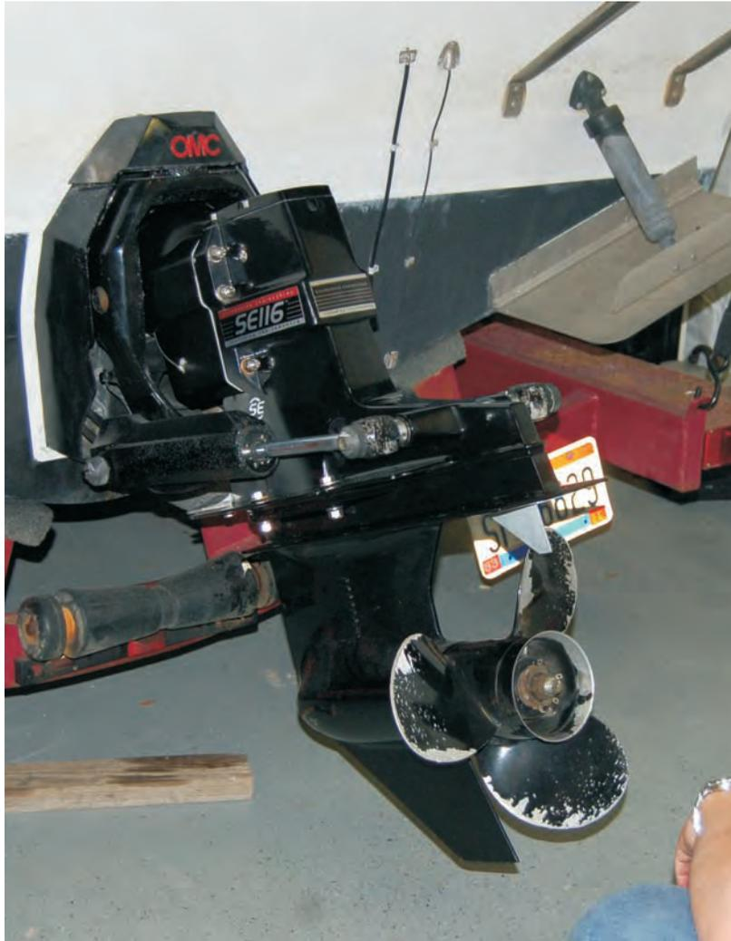
**Step 5.1:** Please assemble and install the drive per the instructions found at <http://www.sterndrive.cc/techspace.htm>. The only notable differences are that you will install the 5/8" plastic spacers between the cylinders and the upper housing to make up the width difference between the SE116™ and the Cobra® drive, and install the plastic spacer guides on the side of the upper housing in the hole provided. Put the bolt head to the outside and the nut on the inside.
