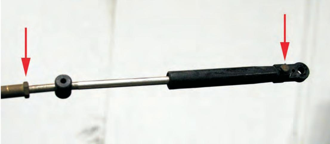
**Step 2.3:** Disassemble the cable end from the intermediate cable. Remove the small set screws and the cable end should slide off. Then loosen the jam nut and unscrew the barrel. Then the shift cable bellows can be removed.
