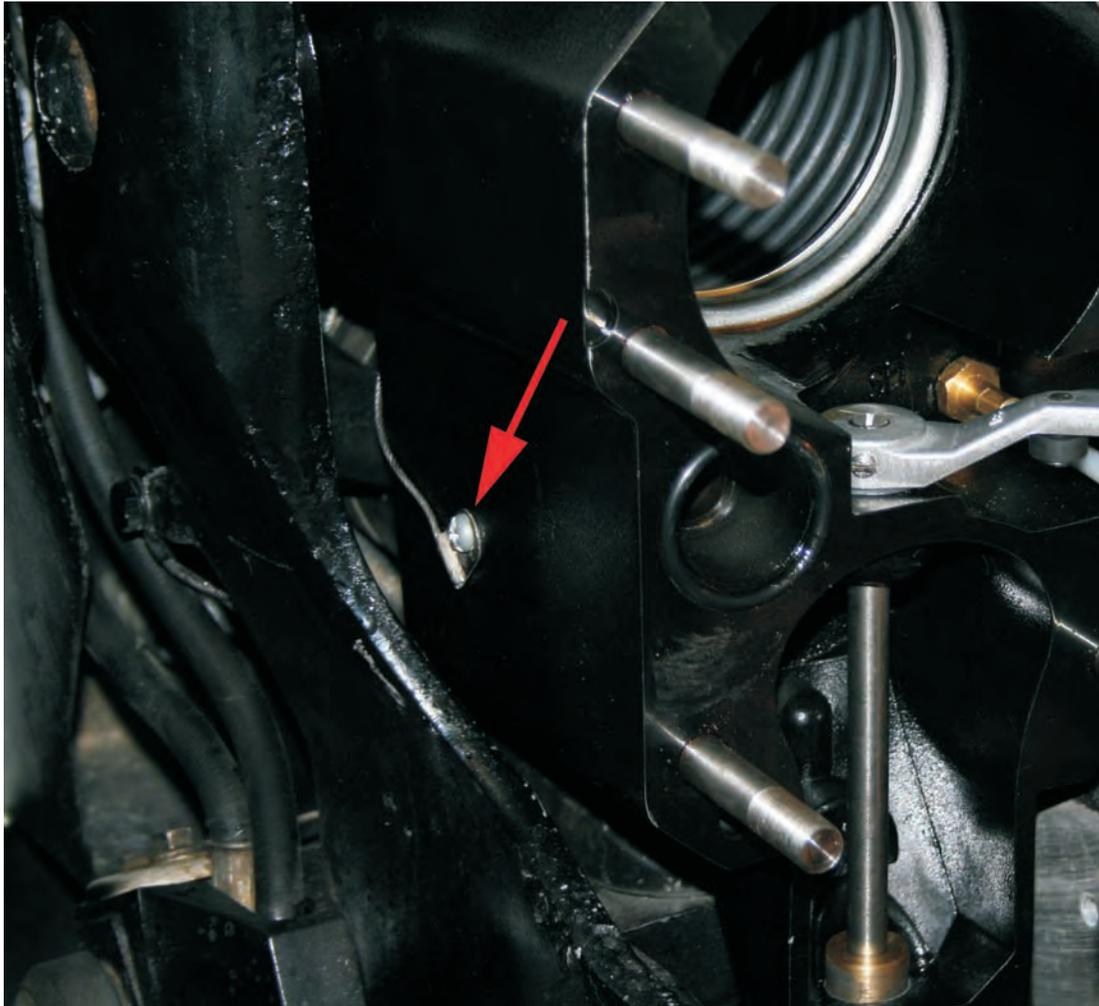
**Step 4.5:** If you had a ground wire attached to the old bell housing, you can now attach it using the small screw to the bell housing attachment spot on the port side of the bell housing near the bottom.
