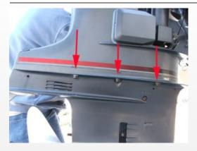
**2.5** Insert the six bolts found along both sides of the gearcase. Using a 14mm socket, tighten them evenly in a circular pattern. Torque the bolts to 29 lb ft.
