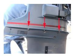
**1.7** Using a 14mm socket or wrench, remove the six remaining bolts holding the gearcase on (arrows). There are three on each side. Remove the gearcase.
