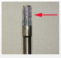
**2.2** Apply grease to the upper splines of the driveshaft. Be sure not to get any grease on top of the driveshaft.
