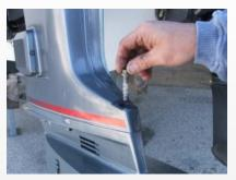
2.7 Insert the trim tab bolt through the access hole. Thread the bolt into the trim tab. Align the trim tab and using a 12mm socket, torque the bolt to 29 lb ft.
