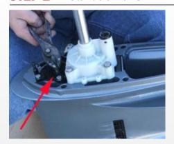
2.1 The gearcase must be shifted into forward gear to match the motor, which was shifted into forward gear before the old gearcase was removed. Using a pair of pliers, turn the shift shaft (red arrow) counterclockwise while turning the propshaft counterclockwise. Turn until the shift shaft stops and the propshaft locks into gear. Be careful not to damage the splines of the shift shaft.
