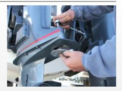
**1.4** (Above) Using a 12mm socket, remove the bolt holding the trim tab in place. Remove the trim tab.
