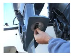
**1.5** (Above) Using a 14mm socket, remove the bolt located under the trim tab.
