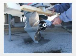
**1.2** Remove the cotter pin securing the propshaft nut. Place a 2x4 between a prop blade and the cavitation plate. Remove the propnut, propeller and thrust washers.
