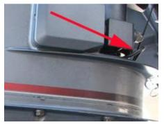
**1.6** Disconnect the pitot hose. There is a hose junction near the lower engine mount (arrow). Some boats do not use the pitot pickup in the drive. Therefore there will be no hose to disconnect.
