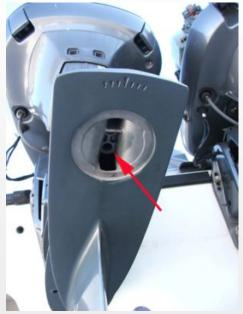
**2.6** Install the bolt under the trim tab (arrow). Using a 14mm socket, tighten it to 29 lb ft.
