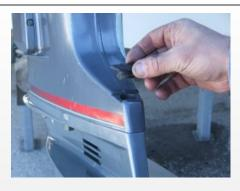
**1.3** (Above) The plug located on the mid-section above the trim tab must be removed to access the trim tab bolt.
