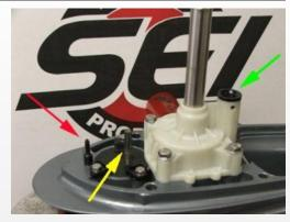
2.3 Apply grease to the splines of the shift shaft (yellow arrow). Smear a small amount of grease into the water tube guide (green arrow). Transfer the pitot nipple from your old drive to the new SE416 gearcase (red arrow). Apply grease to all the bolts used to secure the gearcase to the midsection.
