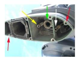
2.4 The new SE416 gearcase comes with new alignment pins already installed. Make sure the old alignment pins are not stuck in the midsection. There are two (red arrows). Insert the driveshaft into the hole in the mid section (green arrow). Raise the gearcase towards the mid section. The water tube in the mid section (yellow
