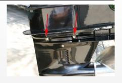
2.9 Install a washer and nut on two of the mounting studs, one on each side, and tighten in an alternating pattern, using a 19mm or ¾" wrench until snug. Check to make sure that the shift shaft is not locked up. If it is not, install the other two nuts and washers and torque all four to 55 lb. ft.
