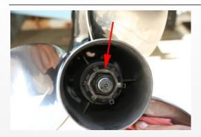
**2.13** Bend three of the tabs of the lock washer down onto the splined washer. If three of the tabs do not line up, tighten the nut slightly more until they do. Do not loosen the nut to align the tabs.
