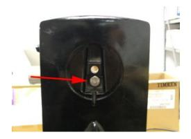
**2.10** Apply grease to the bolt which was removed from under the trim tab. Using a 18mm socket, tighten the bolt to 45 lb. ft.
