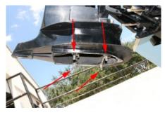
**2.5** Apply grease to the four lower unit mounting studs on the exhaust housing/midsection (arrows).
