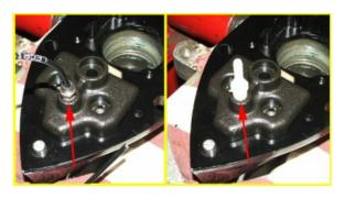
**1.6** The SEI 216 does not include the pitot tube fitting referenced earlier. If your unit uses the gearcase's pitot, the old pieces need to be transferred to the new SEI 216. The two versions are pictured above. Simply unscrew the pieces from your old unit and install onto the SEI 216. If your outboard is a 1999 or older, the housing into which the fitting screws into will look different; however, the threads are still the same.
