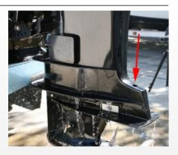
**1.4** Using a ½" socket, remove the bolt holding the trim tab or anode plate. The bolt is accessed through a hole from above (see arrow). Once this bolt is removed, the trim tab or plate drops off of the unit. Under the plate is a mounting bolt which must be removed. Remove it using a 18mm socket.
