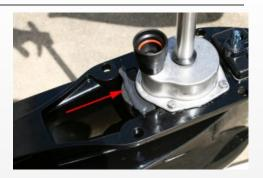
**2.3** Apply a bead of silicone sealant to the top of the filler block (arrow).
