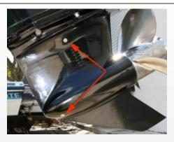
**2.14** Remove the drain plug and fill plug (arrows). Tilt the motor until the cavitation plate is parallel to the ground.
