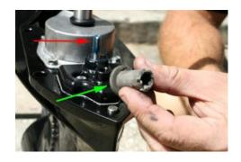
**2.4** Apply grease to the shift shaft (red arrow). Place the shift shaft coupler (green arrow) on the splines of the shift shaft. Place the larger diameter end towards the lower unit. The coupler may be stuck on the end of the upper shift shaft in the exhaust housing. Otherwise, it will be on the shift shaft of the old unit being replaced.
