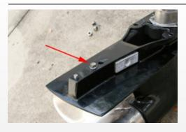
**2.7** Place the trim tab bolt into the rear hole as shown above.
