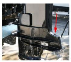
**2.11** Align the trim tab/anode plate and, using a  $\frac{1}{2}$ " socket, tighten the bolt through the access hole in the exhaust housing above it (arrow). Tighten to 40 lb. Ft.
