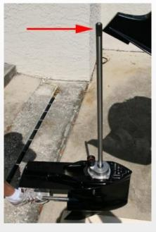
**2.2** Apply a high temp grease to the splines of the driveshaft (arrow). Make sure not to get any grease on the top of the driveshaft.
