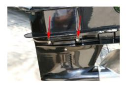
**1.5** Now, the only thing holding the unit on are the four nuts, two along each side (see arrows). Using a 19mm or 3/4" wrench, remove the four bolts. Use an alternating pattern. Be careful when removing the last nut as the gearcase will be free to fall off.
