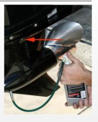
2.15 Install a gear lube pump into the lower drain hole and fill the gearcase until gear lube starts to come out of the upper vent plug (arrow). Reinstall the upper vent plug. Remove the gear lube pump and reinstall the lower drain plug.
