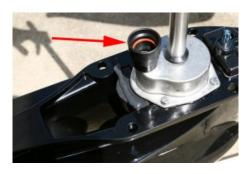
**2.6** Make sure that the water pump guide tube is in place as pictured above (arrow). Apply grease to the orange o'ring.
