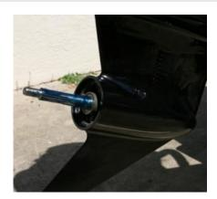
2.12 Apply grease to the propshaft. Install the thrust hub followed by the propeller. Next install the continuity washer on the splined washer and install as an assembly. Next, install the tab washer and finally the nut. Torque the nut to 50 lb. ft.
