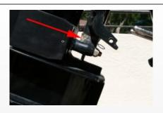
1.3 If your boat uses the lower unit's pitot (speedometer) pickup, you will need to disconnect the tube. The junction of the upper and lower tubes is found at the lower mount (see arrow). On newer models, a quick connect is used. Push in on the junction, and then pull out on the hose. On older models, the junction is a simple hose barb. On these models, cut off the zip tie and pull the hose off of the barb. The model pictured does not use the drive's pitot pickup.
