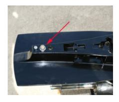
**2.4** Insert the trim tab bolt into the rearward of the two holes at the back of the SE206 unit (arrow).
