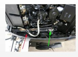
2.13 Slide the splined washer (red arrow) onto the propshaft. Make sure the splines of the washer align with the splines of the propshaft. Slide the tab washer (green arrow) on next, followed by the nut (black arrow). Torque the nut to 50 lb-ft. Bend three of the lock tabs into the top of the splined washer. If three of the lock tabs are not aligned, slightly tighten the nut until they do. Do not loosen the nut to align the tabs.
