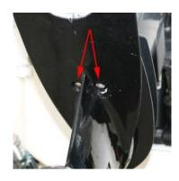
1.7 Using a 5/8" socket, remove the two lower nuts (arrows). Use caution as these are the last two nuts holding the gearcase to the midsection. The unit may fall off if you are not holding it. Remove the unit and set it aside.
