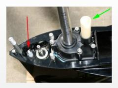
**2.1** Transfer the waterpump quide tube from your old drive to the SE206 unit (green arrow). If your unit uses the gearcase pitot for the boat's speedometer, remove the hose nipple from your old gearcase and transfer it to the new SE206 unit (red arrow).
