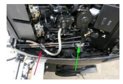
2.6 Remove the engine cowling to gain access to the shift cable. Unclip the cable barrel retainer (red arrow). The upper cable is for the throttle. Move the throttle cable barrel out of the holder and move the cable out of your way. The lower cable is the shift cable. Using a 3/8" socket, loosen the shift cable retainer (green arrow). Remove the cable. Push the retainer all the way towards the front of the boat. The shift rod is now in the forward gear position.
