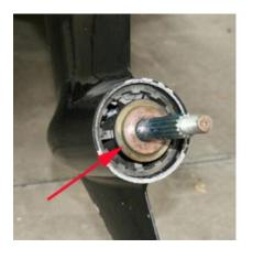
**2.12** Apply water proof grease to the propshaft. Reinstall the thrust hub (arrow). Slide the prop onto the propshaft.
