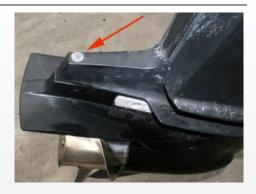
**1.4** Remove the small cover pictured above. Under it you will find the bolt attaching the trim tab. Newer models use a 1/2" hex head, while some older units use a 3/8" allen head. Remove the bolt and trim tab.
