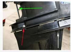
2.8 Place flat washers on the two studs facing upward and hand tighten two nuts onto the threads (red arrow). Check to make sure that the shift rod is not bound up (green arrow). If the shift shaft is bound, slide the shift cable retainer (under engine cowling) back and forth slightly until the shafts align. Once everything is aligned, install washers and nuts on the two studs facing downward (white arrow) and tighten all four nuts in an alternating pattern. Torque the nuts to 50 lb-ft.
