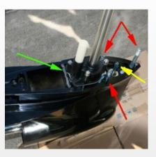
**2.2** Apply silicone sealant to the top of the filler block (green arrow). Apply waterproof grease to the three studs (red arrows). Apply waterproof grease to the splines of the shift shaft (yellow arrow).
