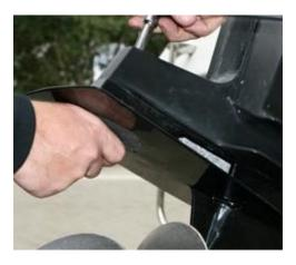
**2.10** Align the trim tab. Using a 1/2" socket, torque the bolt through the access hole, to 34 lb-ft.
