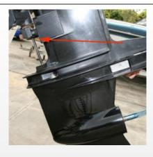
**1.3** Some boats use the pitot pickup in the drive for their speedometer. If your boat does, you will need to disconnect it before removing the drive. It will be alongside the shiftshaft (arrow). The unit pictured above does not use the gearcase pitot.
