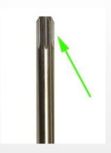
**2.3** Apply grease to the splines of the driveshaft (arrow). Be sure not to get any grease on the top of the driveshaft splines.
