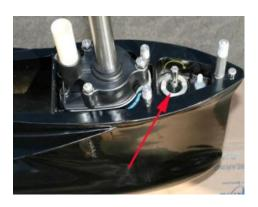
2.5 The gearcase needs to be shifted into forward. Turn the shift rod (arrow) clockwise while turning the propshaft counter clockwise. You will feel the propshaft lock into position when the forward gear position is reached. The shift shaft will no longer be able to turn clockwise as well. In forward gear, when you turn the driveshaft clockwise; the propshaft will turn clockwise.
