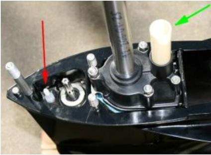
**2.1** Transfer the waterpump guide tube from your old drive to the SE206 unit (green arrow). If your unit uses the gearcase pitot for the boat's speedometer, remove the hose nipple from your old gearcase and transfer it to the new SE206 unit (red arrow).
