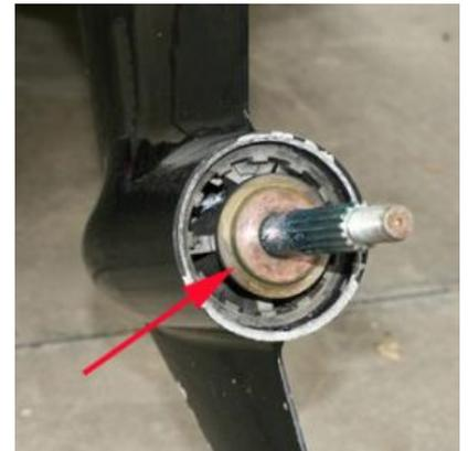
**2.12** Apply water proof grease to the propshaft. Reinstall the thrust hub (arrow). Slide the prop onto the propshaft.
