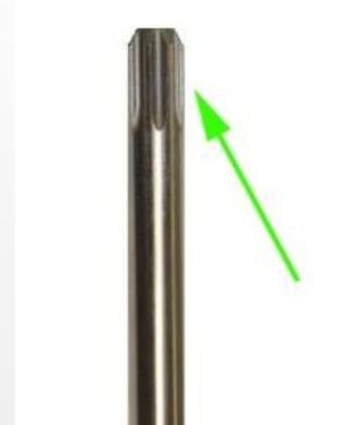
**2.3** Apply grease to the splines of the driveshaft (arrow). Be sure not to get any grease on the top of the driveshaft splines.
