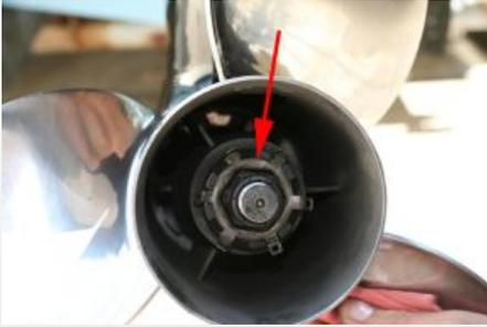
**1.2** Bend the tabs up on the propeller nut lock tab (see arrow). Place a block of wood between the blades of the propeller and the bottom of the cavitation plate. Remove the nut using a 1 1/16" socket. Remove the propeller and thrust washer.
