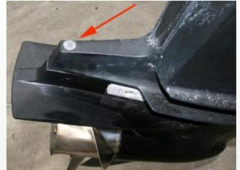
**1.4** Remove the small cover pictured above. Under it you will find the bolt attaching the trim tab. Newer models use a 1/2" hex head, while some older units use a 3/8" allen head. Remove the bolt and trim tab.
