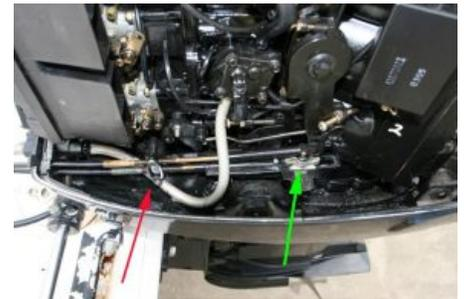
**2.6** Remove the engine cowling to gain access to the shift cable. Unclip the cable barrel retainer (red arrow). The upper cable is for the throttle. Move the throttle cable barrel out of the holder and move the cable out of your way. The lower cable is the shift cable. Using a 3/8" socket, loosen the shift cable retainer (green arrow). Remove the cable. Push the retainer all the way towards the front of the boat. The shift rod is now in the forward gear position.
