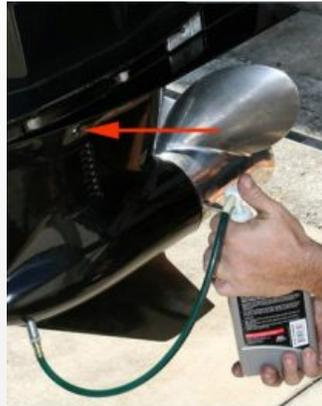
**2.14** Tilt the drive downward until the cavitation plate is parallel with the ground. Remove the lower drain plug and the upper vent plug. Pump gear lube into the unit slowly until lube seeps out of the upper vent plug (arrow). Reinstall the upper vent plug. Remove the pump hose adapter and reinstall the drain plug.
