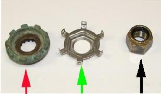
**2.13** Slide the splined washer (red arrow) onto the propshaft. Make sure the splines of the washer align with the splines of the propshaft. Slide the tab washer (green arrow) on next, followed by the nut (black arrow). Torque the nut to 50 lb-ft. Bend three of the lock tabs into the top of the splined washer. If three of the lock tabs are not aligned, slightly tighten the nut until they do. Do not loosen the nut to align the tabs.
