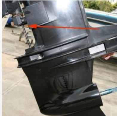
**1.3** Some boats use the pitot pickup in the drive for their speedometer. If your boat does, you will need to disconnect it before removing the drive. It will be alongside the shiftshaft (arrow). The unit pictured above does not use the gearcase pitot.
