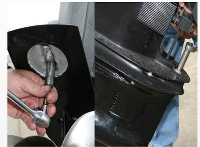
**2.9** Install the bolt under the trim tab and torque it to 41 lb-ft. Install the washer and nut on the stud at the front of the unit and torque it to 50lb-ft.
