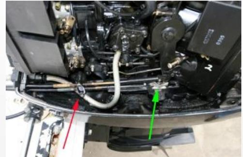
**2.15** Slide the shift and throttle cable barrels into the holder (red arrow). Attach the end of the shift cable to the guide block (green arrow). Tighten down the guide block anchor. Close the latch over the barrel holder.
