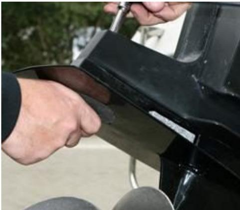
**2.10** Align the trim tab. Using a 1/2" socket, torque the bolt through the access hole, to 34 lb-ft.
