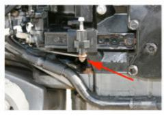
1.12 (Above) Remove the attachment nut for the midsection shift shaft (arrow).
