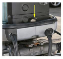
3.5 (Above) Re-tighten the nuts at the front of the cowling, which secure the upper cowling latch (arrow).
