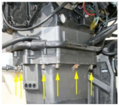
3.1 (above) Place the power head base gasket on the midsection. There are dowel pins, which align it. Make sure all the holes line up. Lower the power head onto the midsection. Apply Loctite 271 to the threads and reinstall the eight mounting nuts and torque them to 45 ft. lbs.
