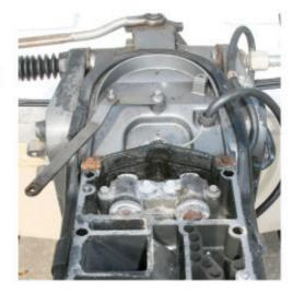
2.3 (Above) Drop the assembled shift shaft back into the midsection in the orientation shown.
