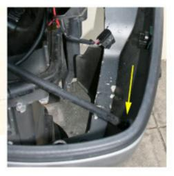
1.11 (Above) Cut the zip-tie holding the tell-tail to the starboard side lower cowling. Pull the hose off of the nipple. The fitting is plastic so be careful not to break it. Remove the lower cowlings and set them aside.
