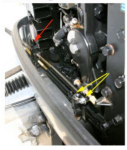
1.2 (Above) Disconnect the battery cables from the battery. Remove the negative side first. On the port side of the engine, use a 10mm socket or wrench and remove the two nuts holding the shift and throttle cables ends (yellow arrows). Slide the retaining clip open (red arrow) and remove the two cables. Slide them out of the cowling.
