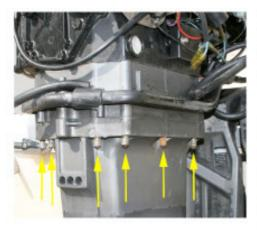
1.13 (Above) Remove the eight nuts holding the power head to the exhaust adapter plate (arrows). Attach a Mercury lifting eye to the flywheel and using a suitable lifting device, lift off the power head.
