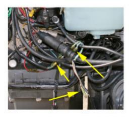
1.7 (Above) Disconnect the wire couplings (arrows) for the trim/tilt system. Make note of the color-coding for use during reassembly. Pull the harness through the cowling. The lower cowling is removed for visibility.
