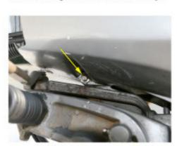
1.8 (Above) Using a 10mm socket, remove the cowling bolt from the port side (arrow).
