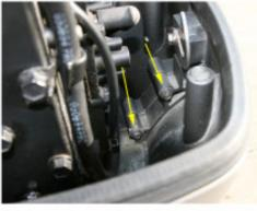
1.9 (Above) Remove the two bolts joining the rear of the two lower cowling together (arrows). Use a 10mm socket or wrench.
