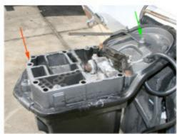
1.15 (Above) Scrape any remaining gasket material and corrosion from the mounting surface on the midsection (red arrow). Lift out the old three-jaw shift shaft (green arrow).
