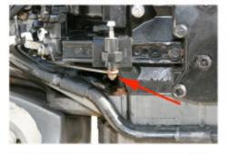
3.2 (Above) Insert a new bushing from the SEI shift shaft kit into the mounting hole of the shift link. Reattach the link to the shift slide (arrow). Tighten the nut until it seats, and then back it off 1/4 turn.
