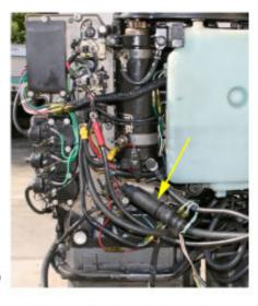
1.5 (Above) Pull apart the wire harness connection (arrow) and pull it through the cowling.
