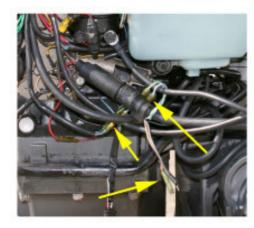
3.7 (Above) Re-connect the electrical connection for the trim / tilt harness (arrows).
