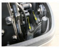
3.4 (Above) Tighten the two rear bolts (arrows). Torque them to 65 in.lbs.
