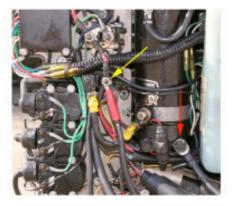
1.3 (Above) On the starboard side of the engine, remove the ½" nut holding the positive battery cable to the solenoid (yellow arrow). Remove the 9/16" headed bolt securing the negative battery cable to the starter mount (red arrow). Slide both cables out of the cowling.
