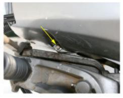
3.3 (Above) Reinstall the two lower cowlings. Remove any corrosion from the mounting bolts and apply waterproof grease to the threads and shoulders of the bolts. Tighten the outer bolt (arrow). Torque to 65 in.
