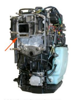
1.14 (Above) Scrape the power head mounting gasket surface (arrow) of any
