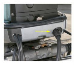
1.4 (Above) Remove the fuel line at the starboard lower cowling quick-connect (arrow). Remove the bolt on switch into the cowling, the inside of the cowling, which holds the quick connect. Pull the fitting into the cowling.
