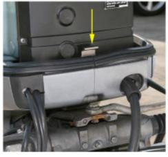
1.10 (Above) Locate the nuts that hold down the front cowling latch (arrow). Loosen the nuts and pull the cowlings apart.
