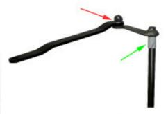
2.2 (Above) Place one of the small bushings in the curved end of the link bar (red arrow). Slide the end over stud of the shift shaft and secure it using one of the nuts from the kit. Place the large bushing on the shift shaft (green arrow). Apply waterproof grease on the bushing. If you are converting a Force, use the original Force link bar.
