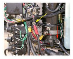
3.9 (Above) Re-attach the positive battery cable to the starter solenoid (yellow arrow). Re-attach the negative battery cable to the starter motor mount (red arrow). Torque the bolt to 14.5 ft. lb.
