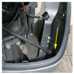
3.6 (Above) Re-attach the tell-tail hose to the nipple in the cowling. Secure it with a new zip tie.
